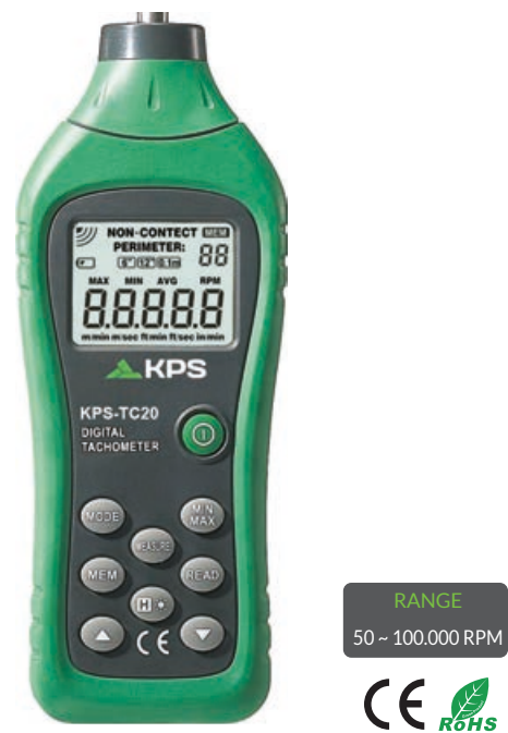
KPS-TC20 Non-contact-type digital tachometer
