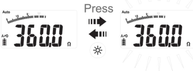
Press the Backlight button to turn the backlight on/off.
