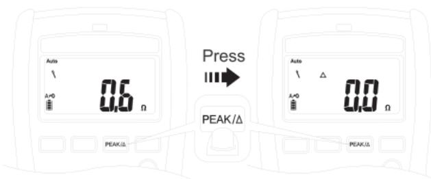
Press the Relative button to enable/disenable this function.
