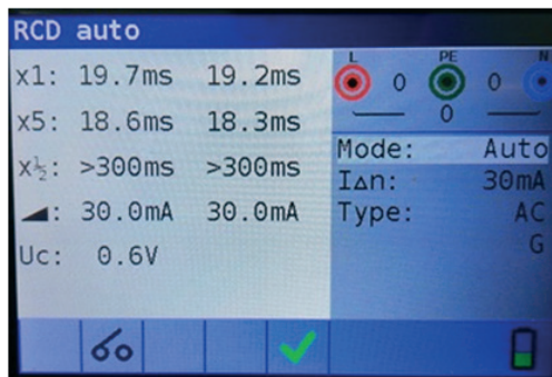
Figure 4 20: Step 8 RCD autotest results
