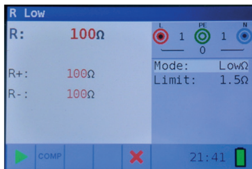
Figure 4 7: Examples of R Low resistance measurement results
