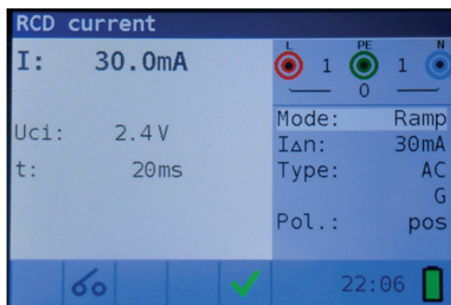
Figure 4 17: Example of trip-out current measurement result
