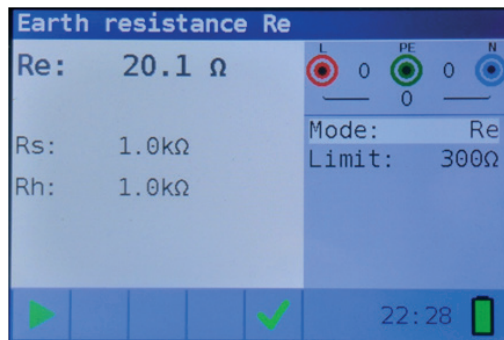
Figure 4 38: Example of resistance to earth measurement results
