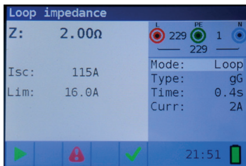
Figure 4 23: Example of loop impedance measurement results
