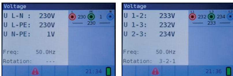
Figure 4.34: Examples of voltage and frequency measurements
