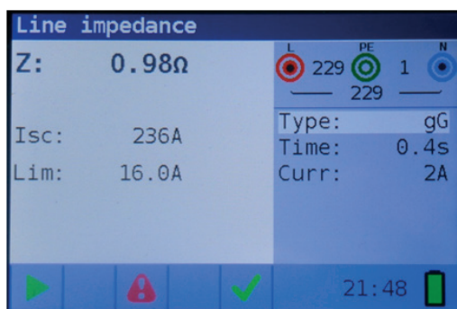
Figure 4 28: Example of line impedance measurement results
